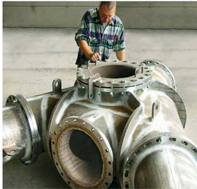
Pressure compensating pipe at the blast furnace; self-supporting structure of KALMETALL W100 30 + 6 hard overlay welding; 450 mm Ø
