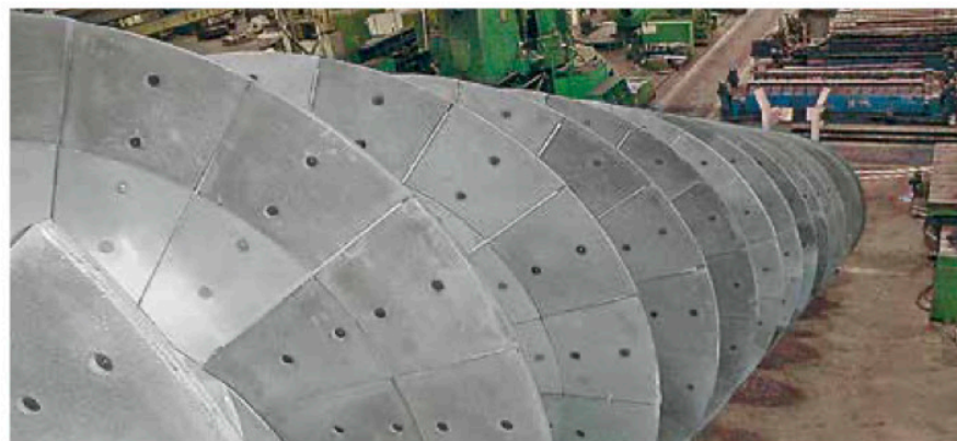
Conveyor screw being part of a slag granulating system; screw flights lined with KALMETALL C155; the screw has a diameter of 1,200 mm
